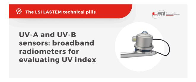
**UV-A and UV-B sensors** are advanced devices in the field of solar radiation monitoring. These broadband radiometers are designed to **measure atmospheric irradiance** in the UV-A and UV-B spectrum, according to WMO standard n.8 chap.7. In this technical pill dive, we explore the distinctive features of these broadband radiometers and their impact in meteorological applications.
