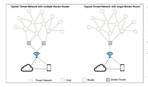
C The **Thread protocol** allows the connection and communication of the Sphensor<sup>™</sup> sensor network to one or more Sphensor Gateways.
