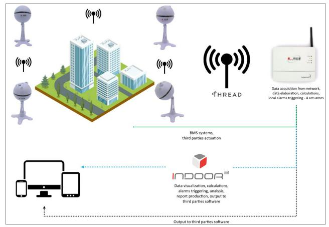
▶ The Sphensor<sup>™</sup> sensors form an indoor sensor network and communicate with each other and with the Sphensor Gateway via 2.4 GHz radio, Thread protocol. The Sphensor Gateway (TXRGB1101) with dual antenna can receive signals from sensors that communicate on the 868 MHz frequency (see Table "Additional sensors integration").
