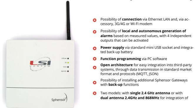
The primary function of the Sphensor Gateway is to decode and route the radio messages arriving from the sensors via the Thread protocol to the MQTT broker reachable via the Ethernet connection and, vice versa, to send the messages coming from the same MQTT broker to the sensors of the net.
