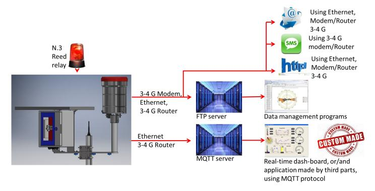
In the picture above there is a general overview of the Alpha-Log data logger data communication/management possibilities. Communication ports/device and data format (Ethernet, RS232-485 ports. HTTP, FTP MQTT protocols), power outputs and alarms by SMS are available in a single device.
