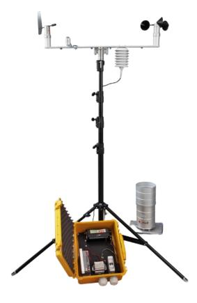
As a portable solution the KME package is equipped with a portable ELF432 enclosure and DYA340 tripod.
