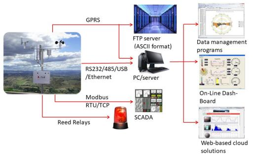
C KME is known for the flexibility of its signal acquisition and data processing system. Produced data is then processed by LSI LASTEM or third-party applications.
