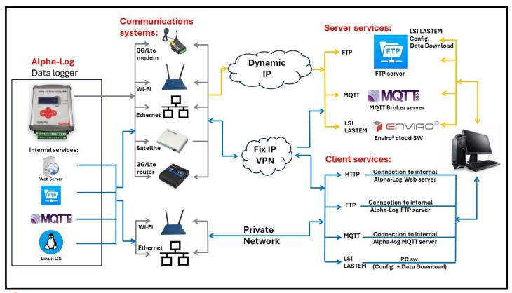
The availability and accessibility of data within the network will depend on the type of communication equipment selected and whether the communication allows for outgoing data only from the data logger (Dynamic IP) or both outgoing and incoming data (Fixed IP, VPN, Private Network).
