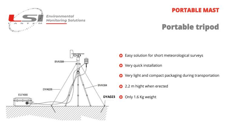
This solution is ideal for short term monitoring campaign using portable equipment. This system is made by a tripod (BVA304) and one H. 80 cm pole (BVA308). For a secure mounting, it is better to use tie-rods (DYA028) and pickets (DYA043).
