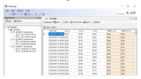
Data browser: measurements listed by device and by surveys (number, date/time of start/end, type).
