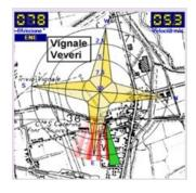
The wind rose is widely configurable in the number of sectors, in the setting of alarms and in the background images
