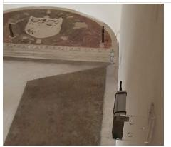
▶ EXP81n sensors range is especially designed for application where advance technical specifications are needed, but even where the monitoring system design must fit the architectural requirements, as in museums. In the picture on the left, two sensors used to monitor Temperature and RH% in the "Last supper" room are shown.
