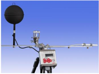
LSI LASTEM developed a high-end instrument range to assess thermal stress (heat stress and cold stress) and comfort. Wet bulb temperature (Tnw) is one important measurement (together with Globe temperature and Air temperature) required by the calculation of the WBGT Wet Bulb Globe Temperature heat index under the ISO7243 standard.
