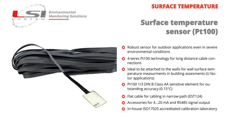
Plate sensor for surface temperature measurements. The compact dimensions allow installation even in small spaces. It can be easily fixed using silicon or adhesive band. Thermoconductive paste can be use to increase the heat exchange.
