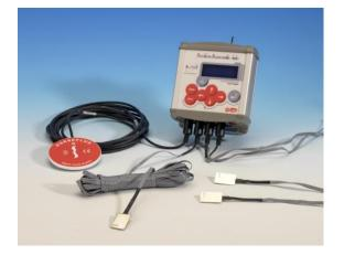
• The EST124 sensor can be connected to the M-Log data logger (ELO009). One of the applications in which it is used, in combination with an ESR240 thermo-flowmeter sensor, is the measurement of walls thermal conductance (U-Factor).
