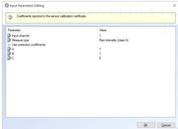
Alpha-Log data logger has the corrective formula for precipitation intensities on board. Following the calibration procedure, parameters a, b and c are obtained to be inserted in the 3DOM configuration software. Thanks to this setting the values recorded by the data logger are already correct and have a relative residual error <± 3% (Class A).
