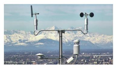
Wind speed sensor can be mounted together with wind direction sensor using the DYA046 coupling bar. On the same coupling bar room for additional sensor as Temperature & RH% and Radiation sensors is available.
