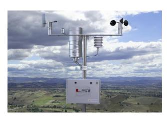
DNA202.1 wind speed sensor can be mounted together with the DNA212.1 wind direction sensor using the DYA046 coupling bar. On the same coupling bar room for additional sensor as Temperature & RH% and Radiation sensors is available.
