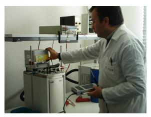
LSI LASTEM is an ISO17025 accredited laboratory for temperature measurements. All sensors manufactured are tested inside our laboratory. LSI LASTEM provides Test report for any sensor and, under request, ISO17025 or ISO9001 calibration certificates (see Accessories list).
