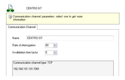
Communication parameters CANNOT be changed (in this case, it's a TCP communication on 192.168.191.101:7001 address), but only the *Rate of interrogation* (in seconds) and the *Interrogation offset* (in seconds) can be changed, that is, the extra time after the interrogation time in order to allow a remote system update. Selecting an item displays a brief description of its function (the icon shows the description of the *Rate of interrogation* parameter).
