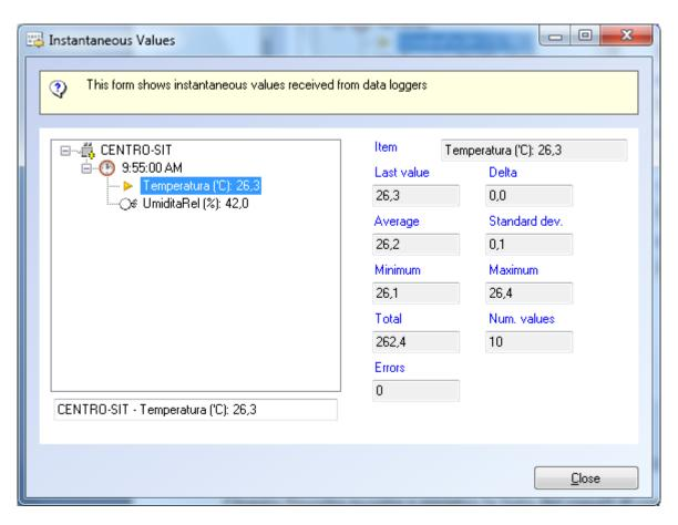
This window shows the list of the communication channels present in the examined configuration, the date/time of the last received data and the list of the available measurements along with their value. Selecting an item from the list makes a detailed description appear on the right of the window.
