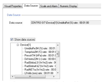
In order to assign/change data sources, communication with *XPanelCommunicator* should be enabled; if enabled, select *Show data source* checkbox to display the data source list and select both *Device* and *Measurement* for their association to the control.
