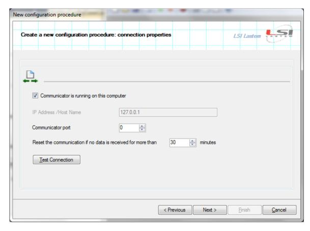
After entering the connection parameters, press the *<Test connection>* button to check for its validity: after - of course – starting *XPanelCommunicator* communication program.
