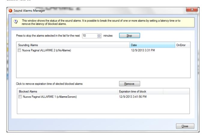
This window displays at the top the indicators list with a sound alarm in progress and at the bottom the one whose sound alarm has been stopped.
