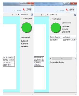
The colored indicator represents the current configuration status; the date of the last received data and the name of the relevant communication channel are shown as well.
