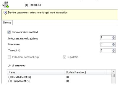
Selecting an item shows a brief description of its function. The details window displays the list of the available measurements as well. "*Instrument needs wakeup*" and "*Is pollable*" options are generally default settings based on the device type and cannot be changed.
