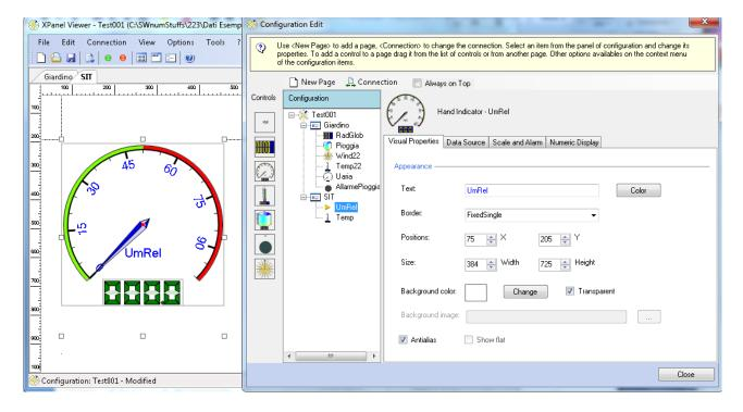
Selecting the *Always On Top>* option, the configuration modification window remains always in evidence with respect to *XPanelViewer* pages.
