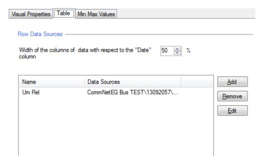
The parameter *Width of the column of data with respect to the Date column* sets the width of the columns of data in percentage to the width of date column. The real size of the columns depends on the width of the control since the table occupies the entire width of the control.
