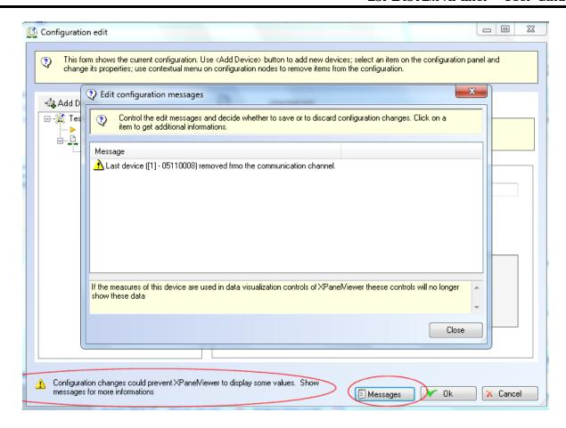
A warning message appears at the bottom of the panel. Selecting the *<Messages>* button allows to check the list of the changes that might need a modification of the corresponding *XPanelViewer* configurations.
