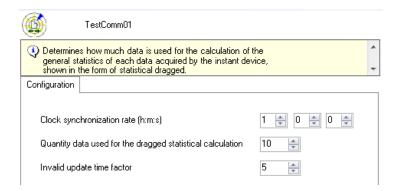
Selecting an item displays a brief description of its meaning (in this case, it explains how much data is used for the dragged statistics).
