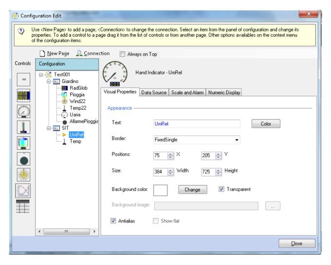
The left section of the window shows the different pages of the configuration and the various controls entered in each page; selecting an item displays its properties in the right section of the window.
