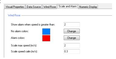
Select *Show alarm when speed is greater than* in m/s; once this value is exceeded, the arrow indicating the wind speed turns the color indicated in the *Alarm colors* box;
