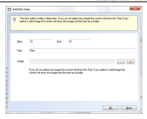
Each state is characterized by a range of values (for integer states use the same value as the *Start* and the *End*), a text and an image optional. If the image is not set the control will display the corresponding text attached to the title, otherwise the control will display the image using the settings described above: in this case the text will be indicated by the tooltip on the control.
