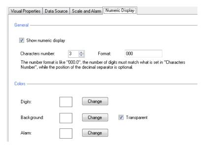
Specifically, set the number format to determine the position of the decimal separator, expressed as "000.0"; the number of digits should correspond to the value set in *Characters number*, while the position of the decimal separator is optional.
