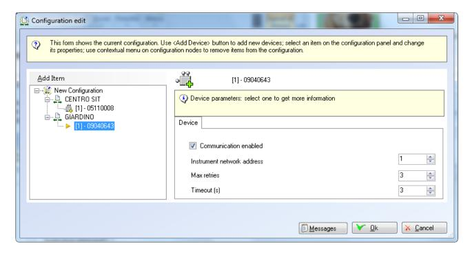
The window displays the list of communication channels and connected devices on the left; selecting an item, a detail is shown on the right allowing the change.
