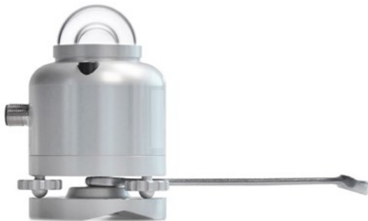
Figure 6.3.1.4 DPA953.1 levelling mount seen from the side: (un)locking with a 10 mm spanner
