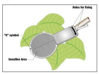
The sensor should be inclined at about 30÷45° with respect to the ground, so as to prevent the stagnation of condensation or rain water on the sensitive surface and simulate the real condition of the leaf type of the cultivation under examination. In case of in-
