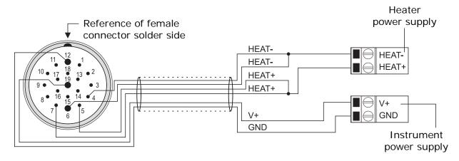
Heating needs 12 Vdc power supply and 6 W power. The heat circuit is switched on below +4 °C. After switching on, the heating is switched off when the temperature exceeds +8 °C.
