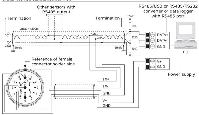
Thanks to RS485 connection, multiple instruments can be connected to a multi-point network. Instruments are connected in sequence through a twisted-pair shielded cable for signals and a third wire for ground.
