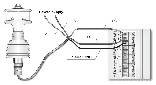
TX+ signal of the anemometer should be connected to +D input of data logger.
