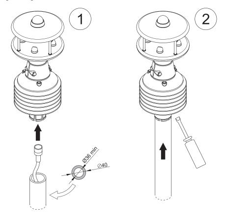
The support mast, having 40 mm maximum outer diameter and 36 mm minimum inner diameter, should be positioned on a stable surface.
