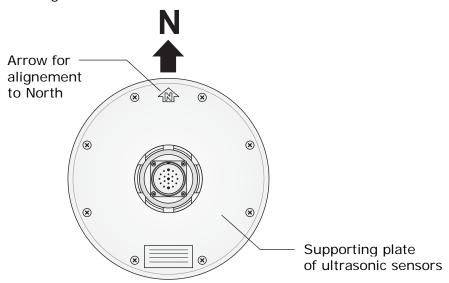
For an accurate alignment, connect the instrument to a PC (see following chapters for communication protocols), then rotate the instrument on its vertical axis until the compass measures  $0.0^{\circ} \pm 0.1^{\circ}$ .
