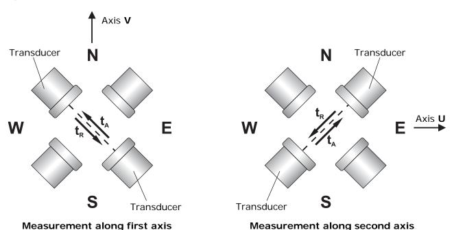
The travel times of the ultrasonic pulses are given by:
