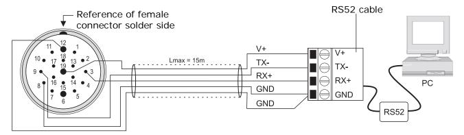
To use the **RS52** cable, the drivers included in the CD-ROM supplied with the instrument should be installed in the PC (see the guide to USB drivers installation in the *Documentation* section of the CD-ROM).
