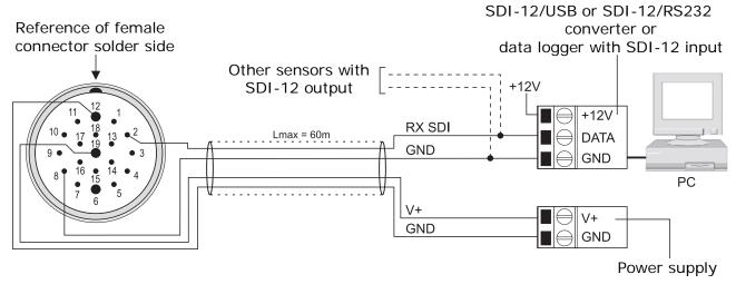
SDI-12 standard has three connection wires: power supply +12V, data line and ground.
