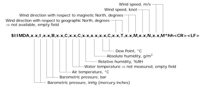
If the instrument model is not equipped to measure some of the quantities indicated in the general format, the relevant fields will be empty and multiple consecutive commas will appear to indicate the missing fields.
