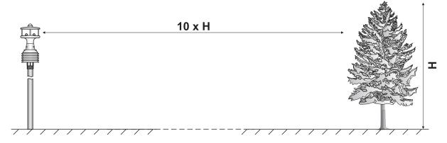
In the presence of close objects, it is advisable to place the instrument at a height of 10 m. For open-space installations, the instrument can be installed using the 3 m tripod **HD2004.20**.
