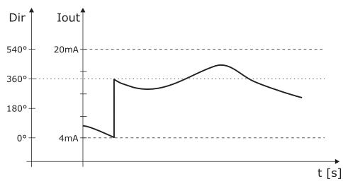
If 539.9° value is exceeded in extended mode, the output goes to the value corresponding to 180°.
