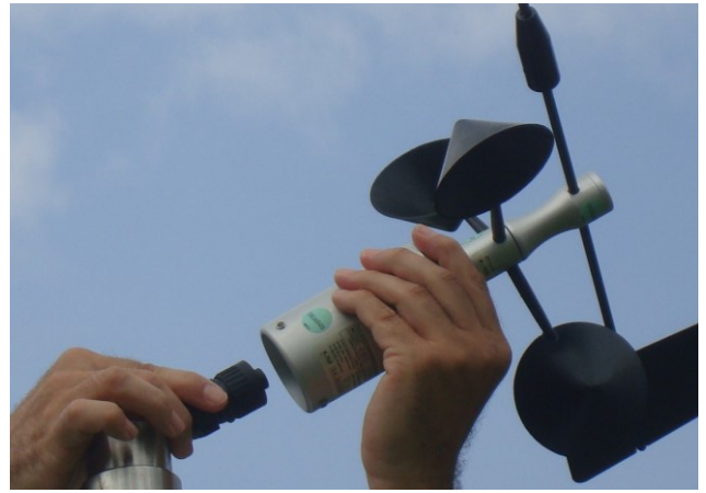
Connect the cable to the sensor.
