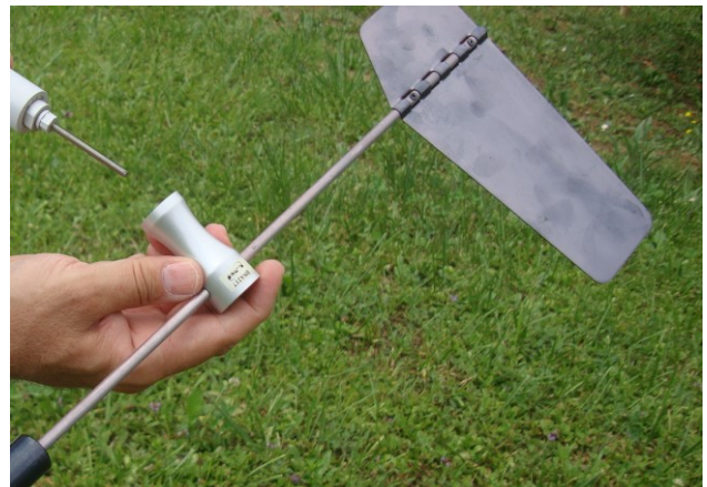
Insert the DNA127 wind vane on the sensor's body. Keep the shank in a steady position and insert the vane until it goes to the nut adjustment.
