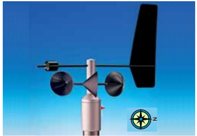
When fixing the sensor in its position on the pole, point the "red nose" to NORTH for orientation.
