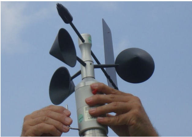
Mount the sensor on the mast and tighten the screw.
