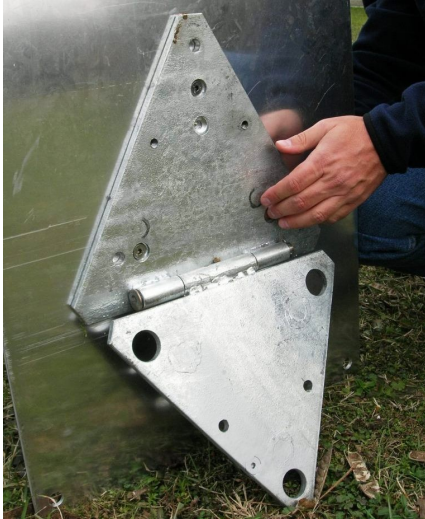
Clamping the base on the DYA320 plate
