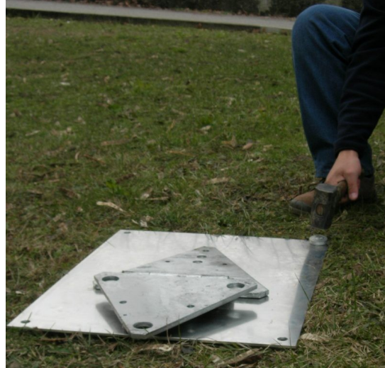
Clamping the DYA320 plate to the ground through pickets
