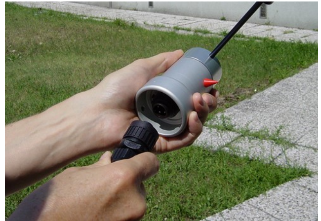
Connect the DWA5xx cable to the sensor. If you do not have the DWA5xx cable but the MG2251 connector, build the cable as indicated below.
