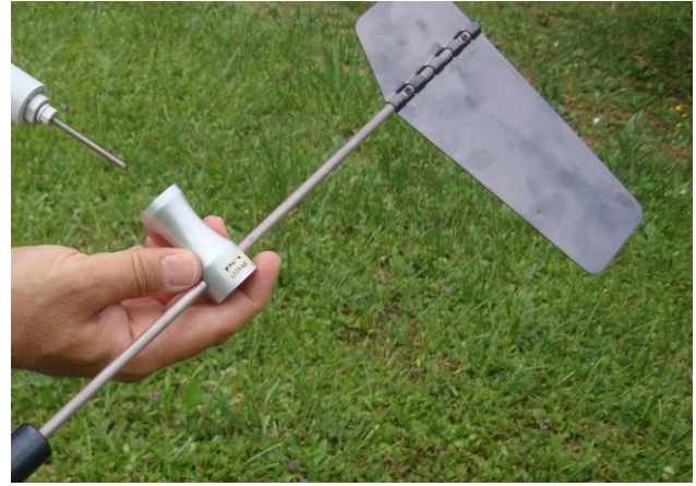
Insert the DNA127 wind vane on the sensor's body. Keep the shank in a steady position and insert the vane until it goes until the nut adjustment.
