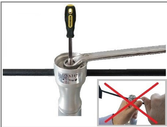
Insert the washer and nut on the threaded shaft; then tighten with a wrench while holding the shaft with the screwdriver. ATTENTION! Do not tighten the nut by holding the windvane with your hand to prevent that the sensor loses its setting.
