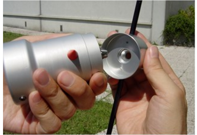
Insert the DNA218 wind vane on the sensor's body. Take care to centre the wind vane's notch with the tooth on the sensor body's rotating cone.
