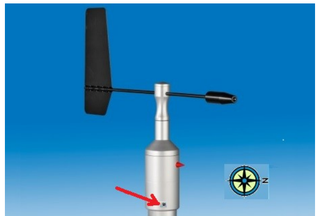
Mount the sensor on the mast and tighten the screw. When fixing the sensor in its position on the pole, point the "red nose" to NORTH for orientation.
