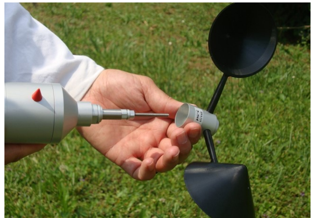
Mount the DNA124 rotor on the combi sensor's body.
