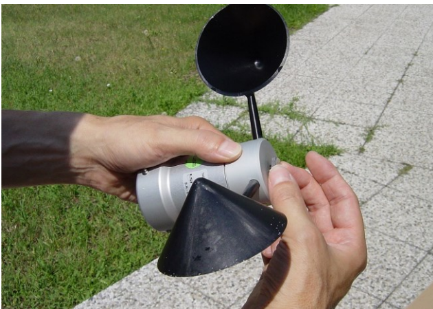
Tighten the screw of the rotor. Attention: don’t leave the sensor in outdoor operation without its rotor.
