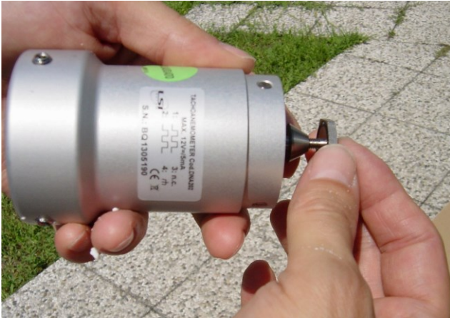
Unscrew the screw from the shaft thread.
