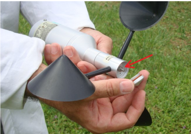
Tighten the screw of the rotor (indicated by the arrow) and the cover. Attention: don't leave the sensor in outdoor operation without its rotor.
