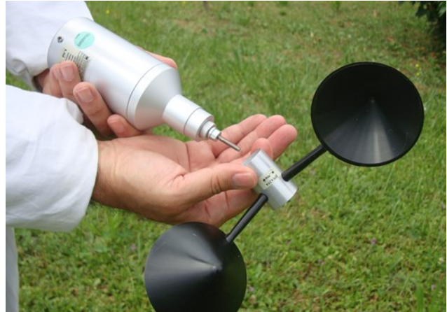
Mount the DNA204 wind rotor on the sensor's body. Keep the shank in a steady position and insert the rotor until it goes to the nut adjustment.
