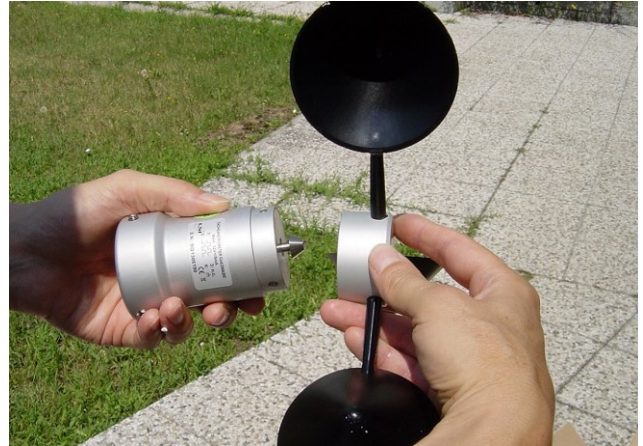
Mount the DNA207 rotor on the sensor’s body.
