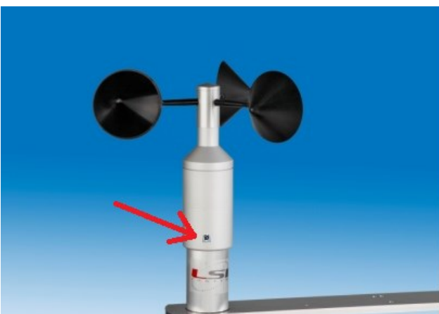
Mount the sensor on the mast and tighten the screw (indicated by the arrow).
