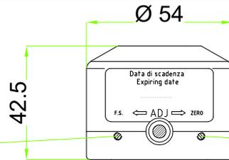
FORO PER REGOLAZIONE FONDO SCALA / Hole for full scale adjustment
