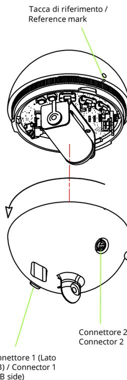
The sensor uses a rechargeable battery placed on the underside of the board located inside the sensor. It can work connected to the power supply via micro-USB cable. In case of battery replacement:
