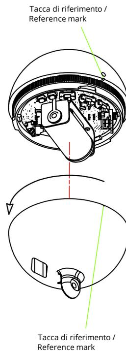
1. With one hand, hold the upper half sphere and the diffuser ring steady and with the other hand unscrew the lower half sphere by turning it counterclockwise.
