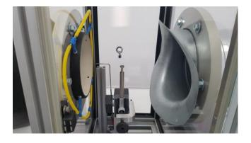
LSI LASTEM is an ISO17025 accredited laboratory for air speed measurements. All sensors manufactured are tested inside this laboratory. LSI LASTEM provides Test report for any sensor supplied and on request, ISO17025 or ISO9001 calibration certificates (see Accessories list).
