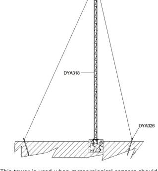
This tower is used when meteorological sensors should be mounted ten meter from the ground. The tower is equipped with accessory to be fixed on concrete plinth. This equipment is very light and handy. The tower comes divided in three sections of 3 m each, on top there is a Ø 50 mm pole. Tower pull down is made using a hinge placed on its base.
