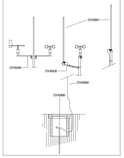
Lightning rod can be mounted on the top of  $\emptyset$  50 mm masts or by means of the DYA058 lateral bar, on the lateral side of them. It is better to mount lightning rod on higher and separate masts than on the one where the equipment is installed. The system is made by the following units:
