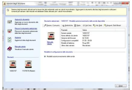
○ GIDAS-TEA includes a functionality that, according to the available sensors, sends the most appropriate configuration to the data logger (M-Log) to carry out microclimate surveys. It also includes a specific function for data download without the use of 3DOM
