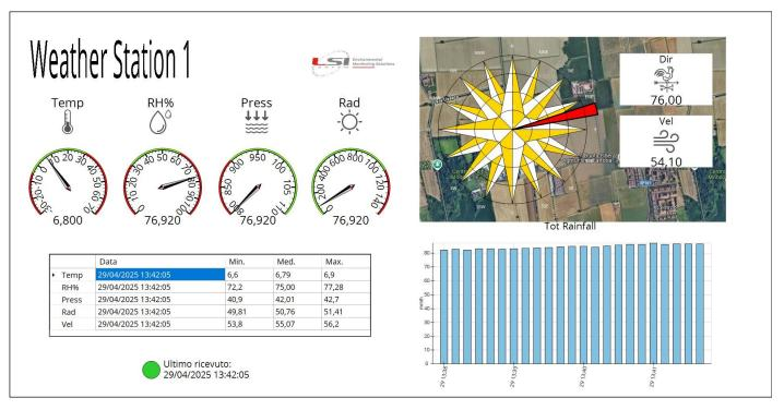
Example of a control panel, in which the following dynamic objects are positioned: Icons of quantities, graphs, compass rose, tables with statistical values, communication status. The compass rose is largely configurable in the number of sectors, alarm setting and background image
