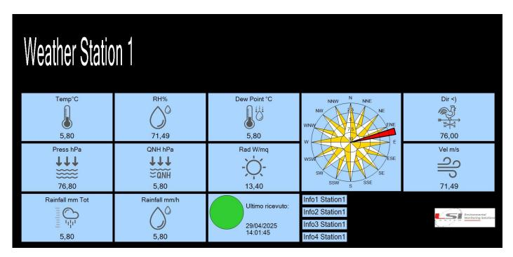
Titles and images can be added on the control panel, it is also possible to configure the navigation through the various pages: manually selectable through labels or with automatic scrolling
