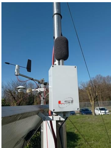
🔴 Outdoor installation on pole with special mounting plate
