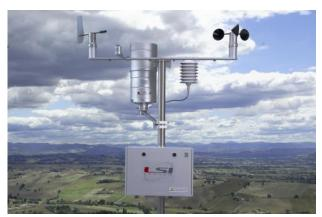
DNA202.1 wind speed sensor can be mounted together with the DNA212.1 wind direction sensor using the DYA046 coupling bar. On the same coupling bar room for additional sensor as Temperature & RH% and Radiation sensors is available.
