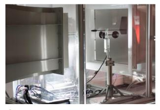
LSI LASTEM is an ISO17025 accredited laboratory for air speed measurements. All sensors manufactured are tested inside this laboratory. LSI LASTEM provides Test report for any sensor supplied and on request, ISO17025 or ISO9001 calibration certificates (see Accessories list).
