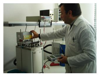
LSI LASTEM is an ISO17025 accredited laboratory for temperature measurements. All sensors manufactured are tested inside our laboratory. LSI LASTEM provides Test report for any sensor and, under request, ISO17025 or ISO9001 calibration certificates (see Accessories list).
