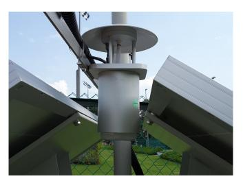
Outdoor measurement of the wet bulb temperature finds its most typical application in the calculation of the WBGT index (ISO 7243) when continuous outdoor monitoring is required. In these cases, small sensors with little water capacity and inadequate solar shields are not suitable. The DMA121A and DMA122 sensors are the "meteorological" solution for this kind of measurement.
