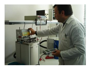
LSI LASTEM is an ISO17025 accreditaded laboratory for air temperature measurements. All sensors manufactured are tested inside our laboratory. LSI LASTEM provides Test report for any sensor supplied and on request, ISO17025 or ISO9001 calibration certificates (see Accessories list).
